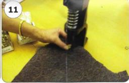
Put the fabric on top of the EYELET and the STUD over the fabric. Align them by holding the stud with your fingers. Press handle as before.
