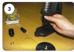
Take the SOCKET DIE and screw it to the threaded rod.
