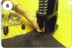
Put fabric on top of the CAP and place SOCKET over the fabric. Align the two pcs. by holding them with your fingers.
