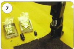
Press the handle of the W-1 machine down to set the CAP and the SOCKET together.
