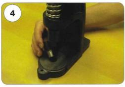
Slip CAP DIE into the bottom hole of the machine.
