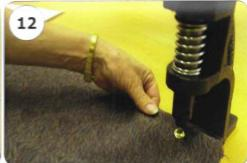
Release the handle and remove fabric. STUD and EYELET has been set.
