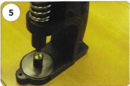
Lay down the CAP on the bottom die as shown in the picture.
