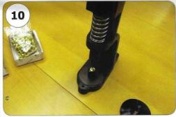
Lay down the EYELET on the bottom die as shown in the picture.
