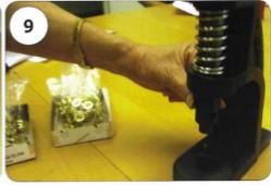
Replace CAP & SOCKET dies. Insert the STUD DIE to the threaded rod and slip EYE-LET DIE to the bottom hole of machine.
